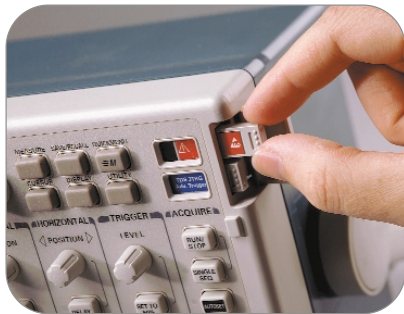
► Application module being installed.
